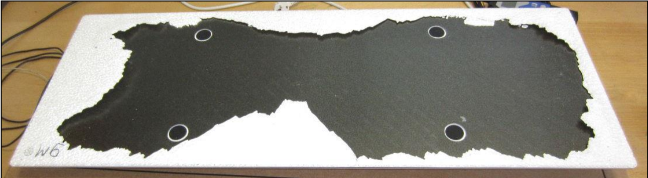
View of the heater with pieces of broken glass fallen off
