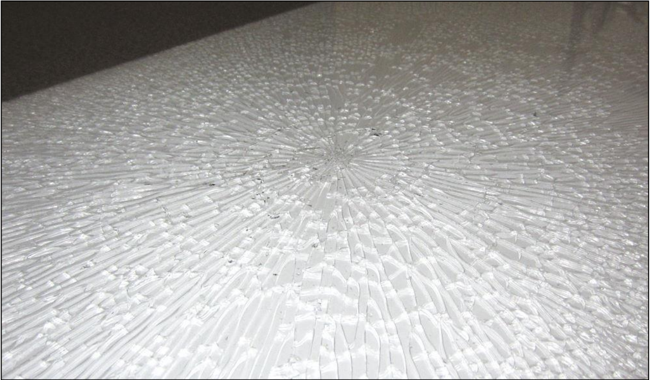
Cracks of the tempered glass (front panel) after 2.0 J blow test
